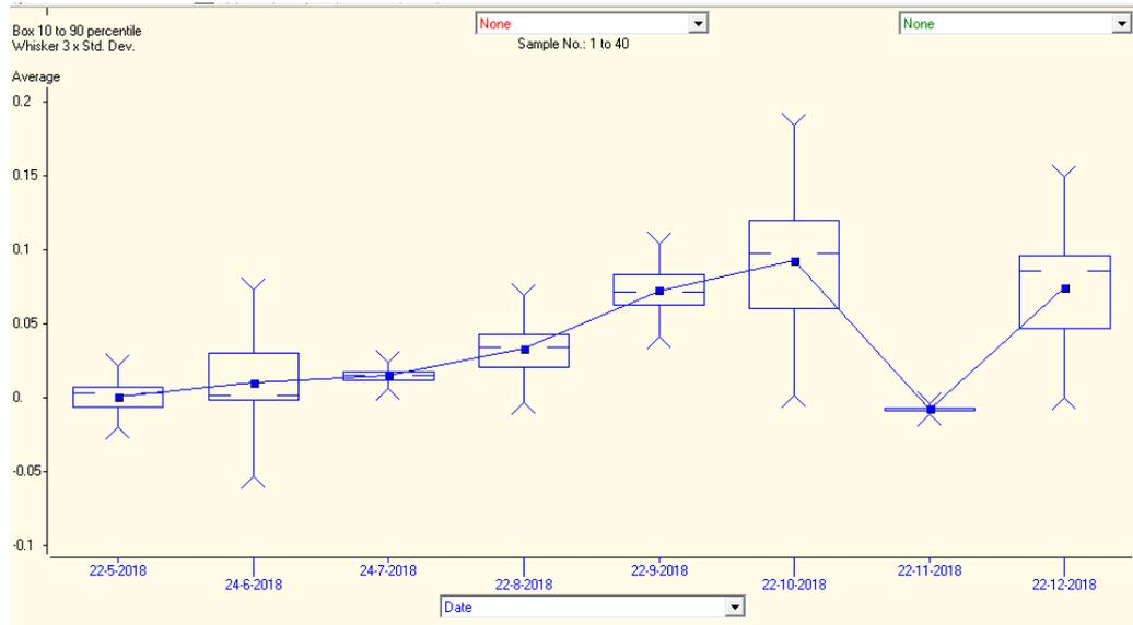
Figure 10: Box and whisker of Calibration results 12171 caliper
