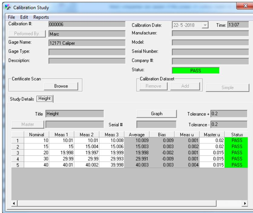
Figure 1: Example screen of a calibration study with 5 nominals
