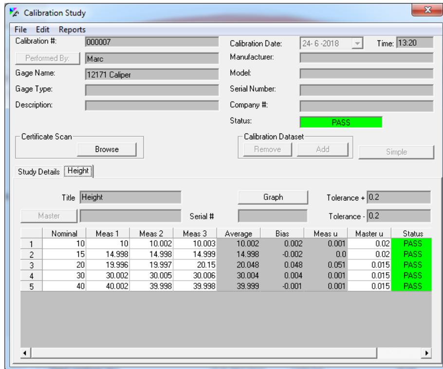
Figure 6: Calibration results in June without applying SPC
